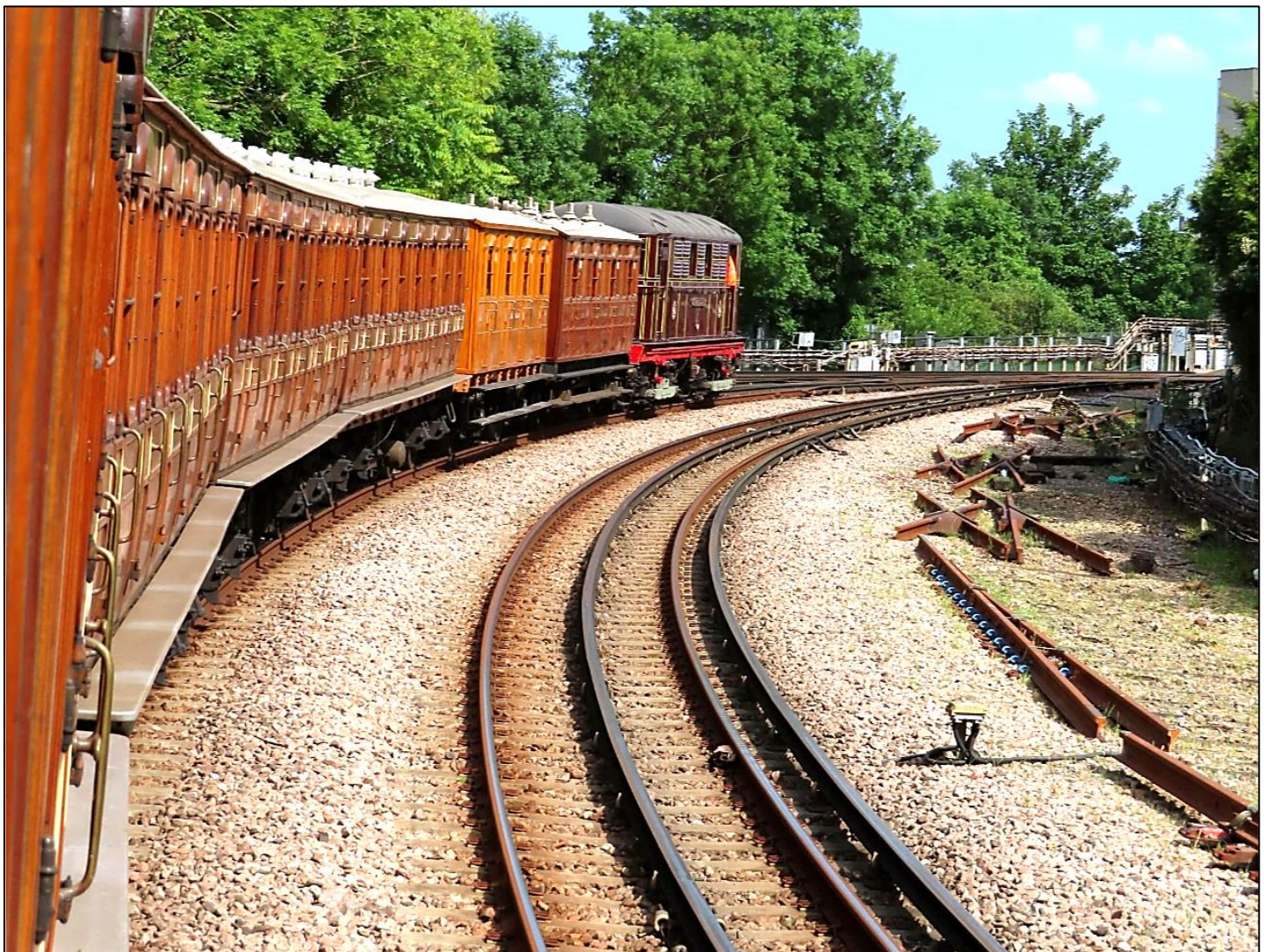
Above: On the eastbound and approaching Hanger Lane Junction after leaving Ealing Broadway with Sarah Siddons leading. Note the footboards that were common on handworked door stock.
